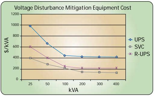
Figure B -- The cost per kVA of traditional and newer technology voltage variation solutions.
